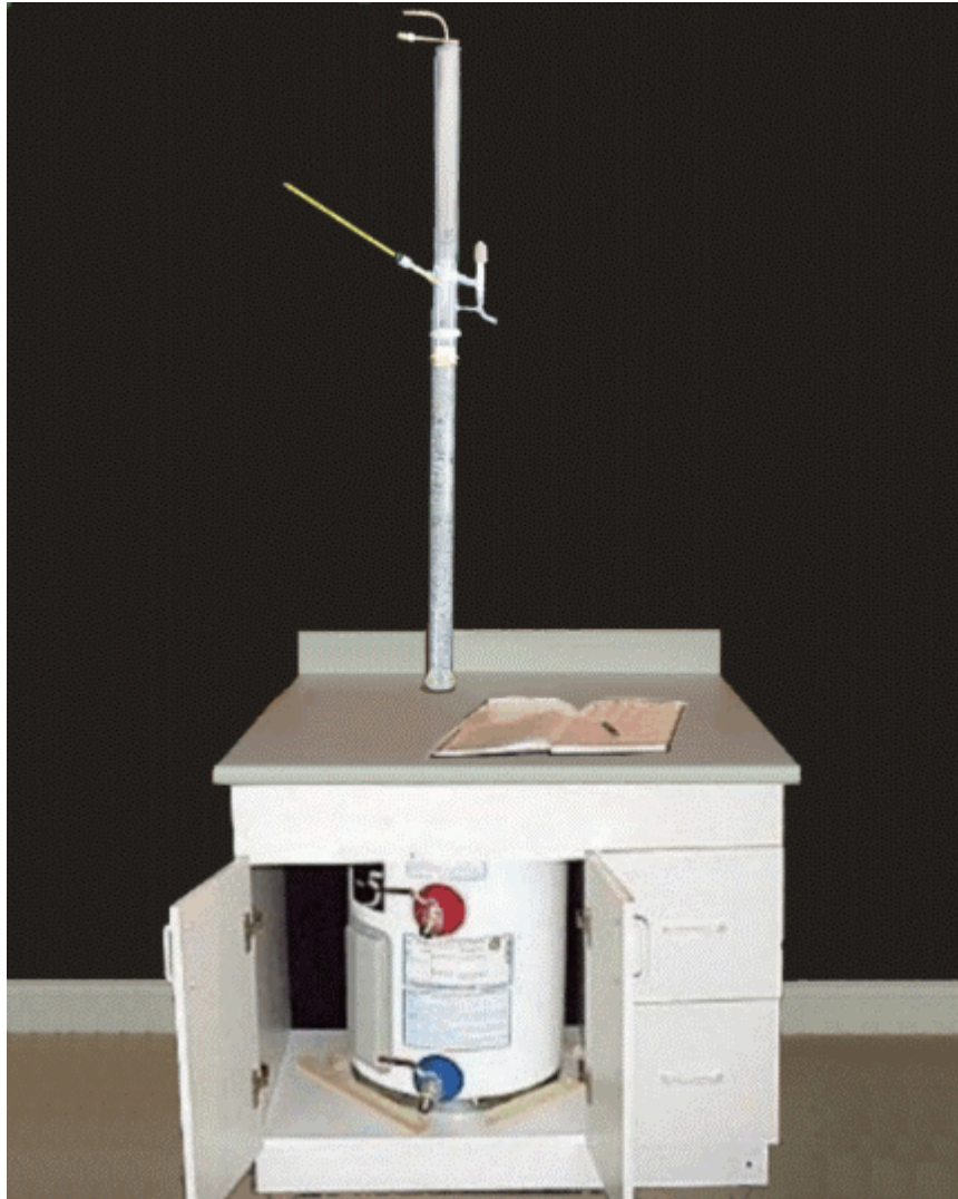
Figure 9. Suggested arrangement for cabinet-mounted still
